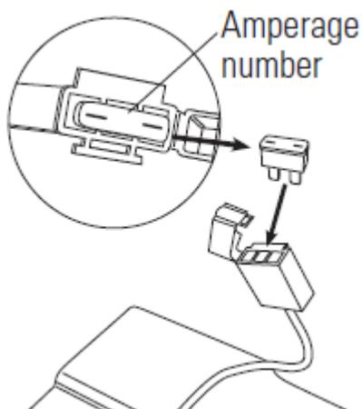
3. Remove any fuse that is damaged or burnt out and replace with a new one of equal amperage.
