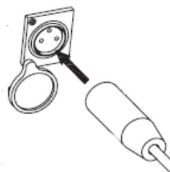
**1** Turn **OFF** power switch before charging. Plug charger into the charger port on the electric motor bike.
