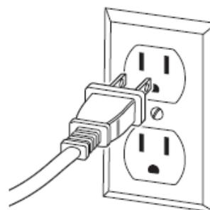
**2** Plug the charger plug into a wall outlet. If the lights on the charger do not light up, check the power to the outlet. If necessary, try a different outlet.
