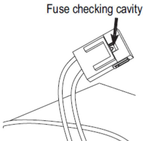
2. Check the fuse to see if it has burnt out. If the fuse is damaged, open the fuse cover.
